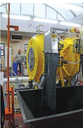
Biosolids, fed into two rectangular channels, slowly moves between two parallel revolving stainless steel filter plates. Filtrate passes through these slotted, wedge wire plates as the flocculated material advances. Dewatering continues until the material reaches a tapered restriction zone at the outlet of the press. An adjustable two-piece pneumatic restriction plate squeezes the material into the final dry cake.
