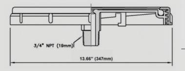
DESIGN FLOW: 2.5 - 5.0 SCFM (4.2 - 8.3 Sm<sup>3</sup>/hr) FLOW RANGE: 0 - 12 SCFM (0 - 20 Sm<sup>3</sup>/hr) ACTIVE SURFACE AREA: 0.700 ft<sup>2</sup> (0.065 m<sup>2</sup>)
