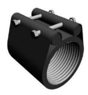
Expansion Joints are available in a positive locking design or in flexible PVC with a stainless steel shell. SSI recommends the flexible expansion joints for disc installations and the positive locking type for tube diffuser projects
