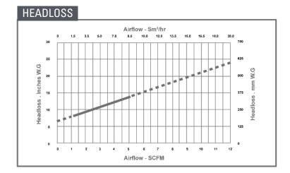
diffuser. AFD350 has an even lower headloss than AFD270, often resulting in the highest SAE (kgO2/kWh) when compared to other fine bubble diffusers.
